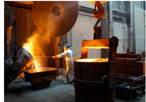
Intensive and separate extraction in the magnesium treatment
