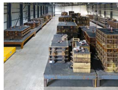
System-controlled cooling house with ventilation and exhaust air extraction system and heat recovery
