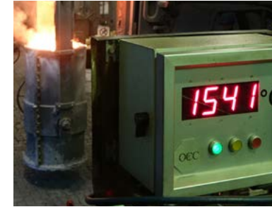
Temperature monitoring of the molten mass
