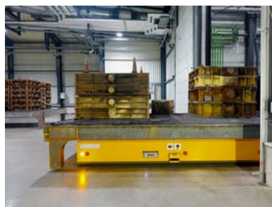
Automatic transport logistics with unmanned floor conveyors
