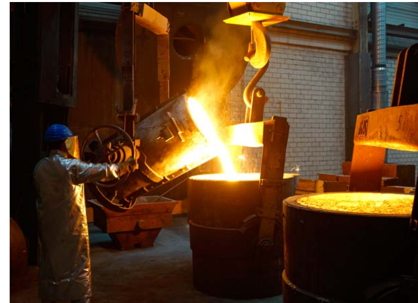
Recasting the magnesium-treated molten mass into the casting ladle
