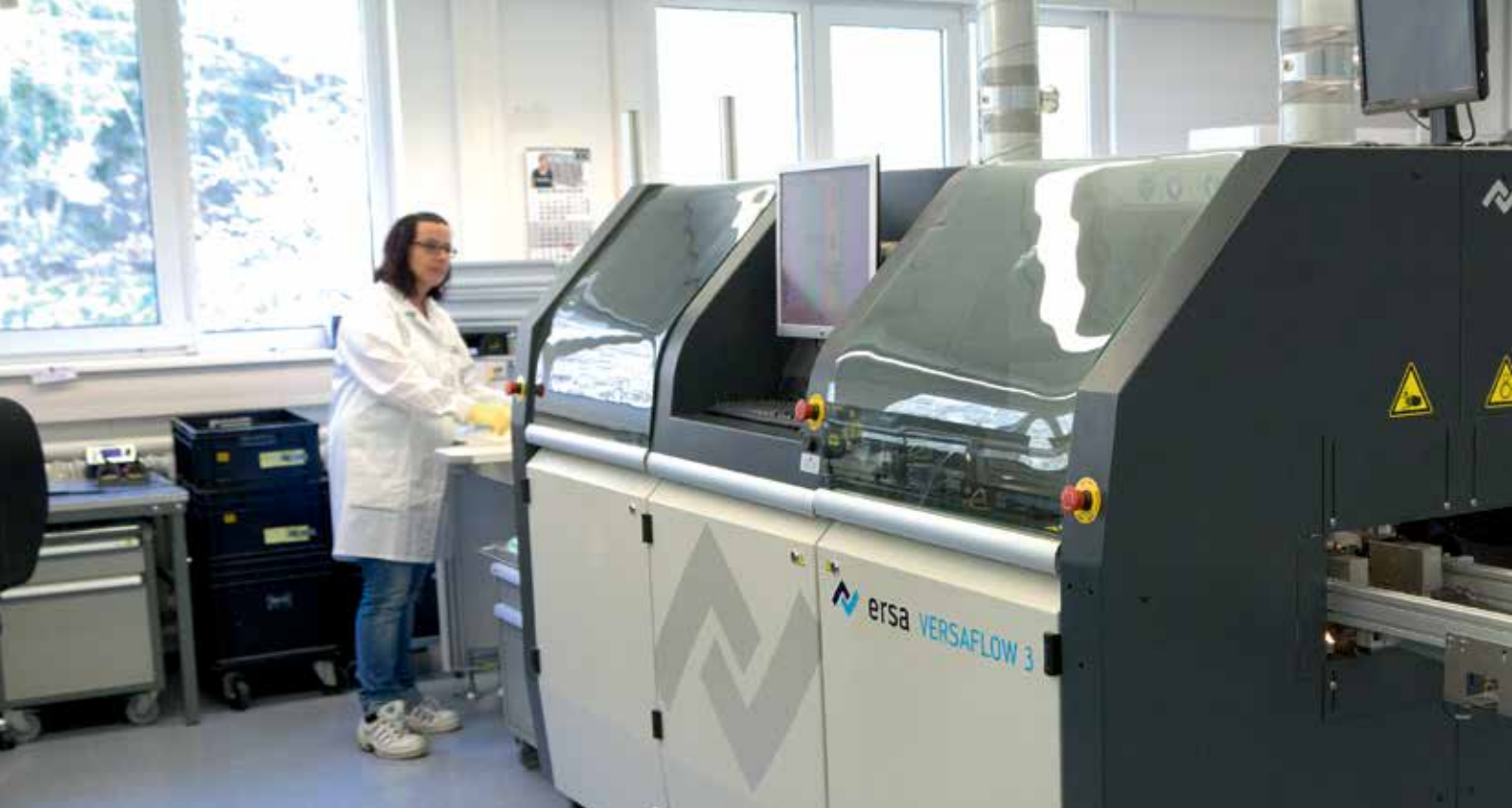
With two crucibles optimally equipped for highest possible throughput: ErsafLOW 3/45 in the HUND production.
