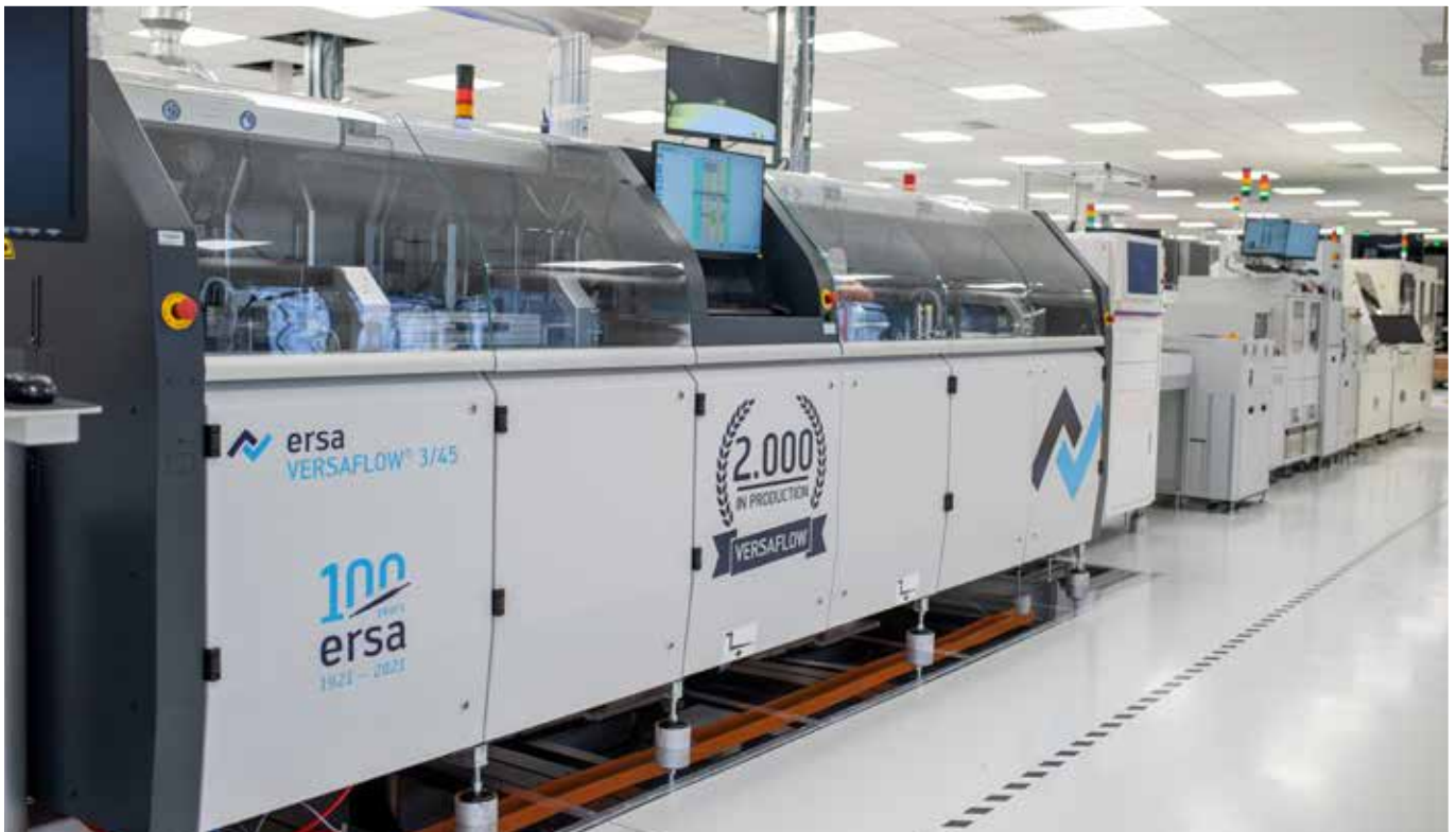
Fits seamlessly into the Flex electronics production in Zalaegerszeg: the anniversary machine VERSAFLOW 3/45, which is already the 26th Ersa selective soldering machine at the Hungarian site; Photo: Flex Ltd.
