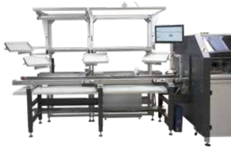
Dual workstation system integrated to Kurtz Ersa Automation product carrier circulation system. Integrated vision-based worker assistance system, combined with goods carrier release at IO inspection result
