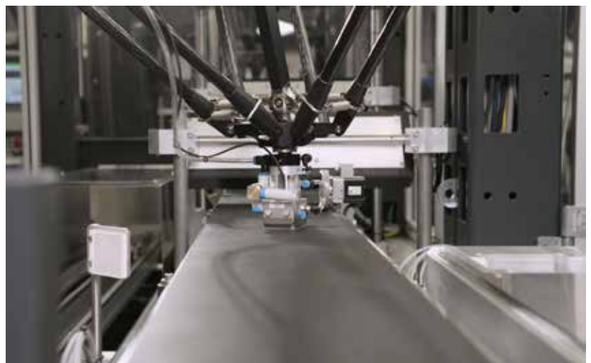
Position-corrected removal of components from the conveyor
