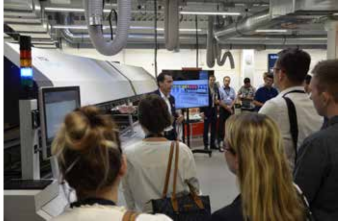
Hands-on unit at the HOTFLOW THREE: Ersa Product Manager Michael Haas presents the reflow soldering system, which scores among other things with its three-stage cleaning system
