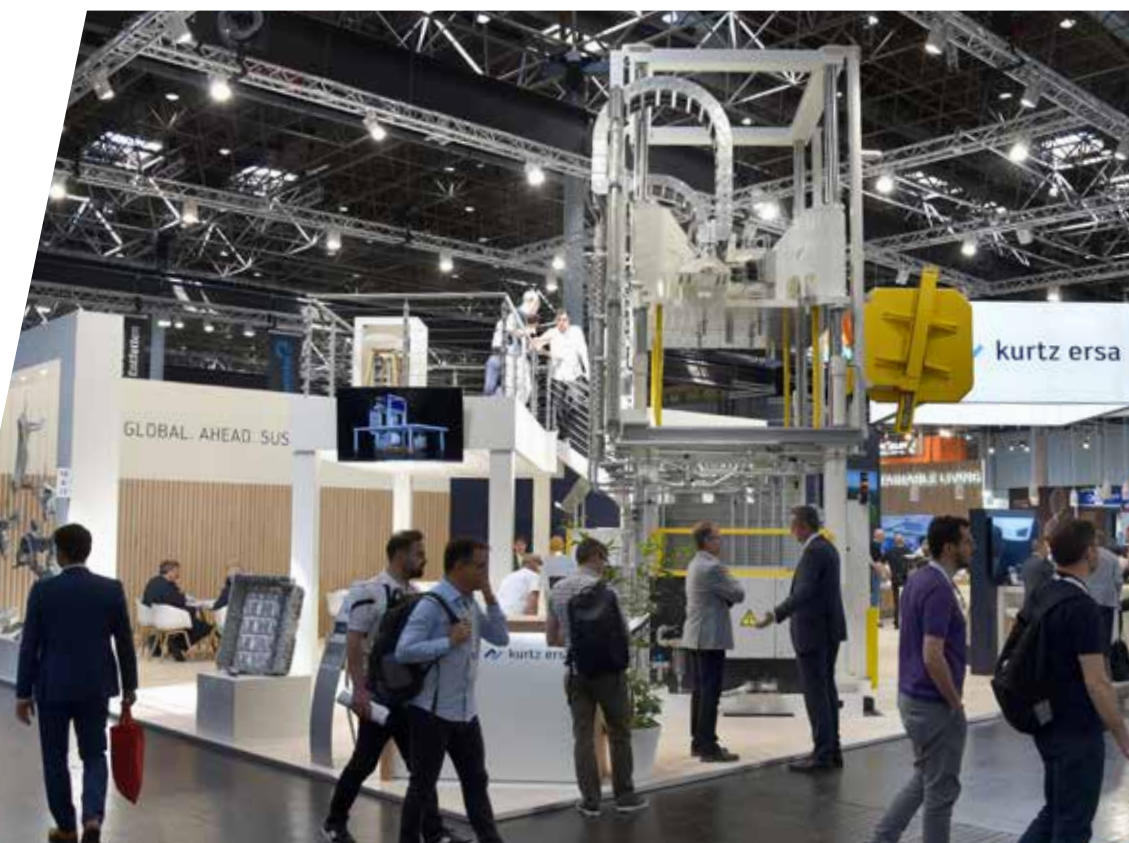
Centerpiece of the booth and the Kurtz answer to the GIGA casting trend: the Kurtz low pressure casting machine with more clamping area, multiple riser system, large furnace capacity and high closing and opening forces
