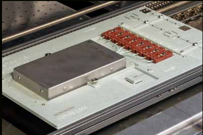
The new horus® Professional Temperature Profiling measuring electronics can also be used with existing measuring boards and guarantees reliable thermal processes
